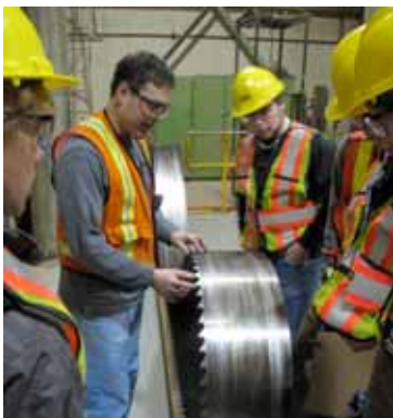
Paul Bergeron, Head Filer at Canfor's PG Sawmill describes how band saw teeth are filed to exacting specifications.
